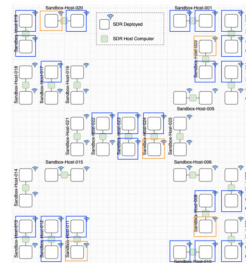
Fig. 5. ARA sandbox, with gNBs and UEs marked in orange and blue colors respectively
