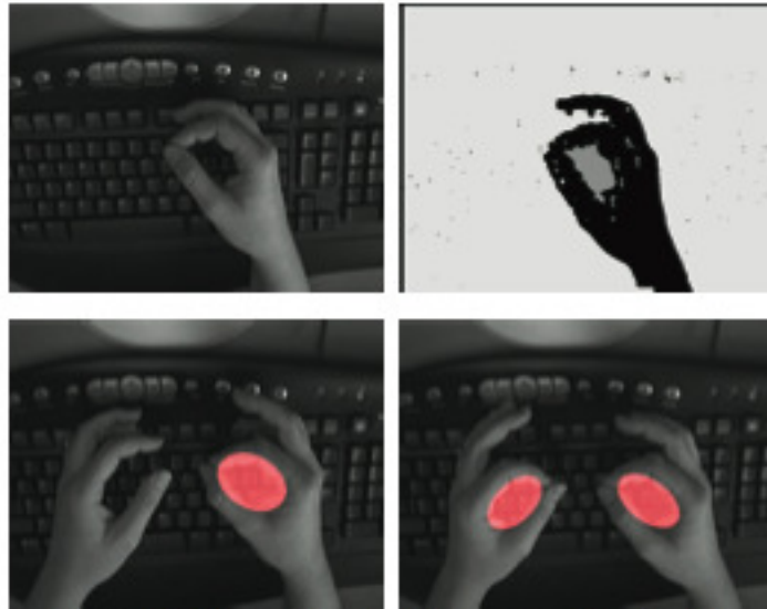
Figure 2: Upper left: Typical image of hand with thumb and forefinger together, acquired from camera above the keyboard. Upper right: Image segmentation indicates background pixels. The hole formed by the thumb and forefinger is detected as a distinct connected component (shown here darker in color). Bottom left: Ellipsoidal model of hole component for the closed hand, shown in red. Bottom right: two hands are detected.
