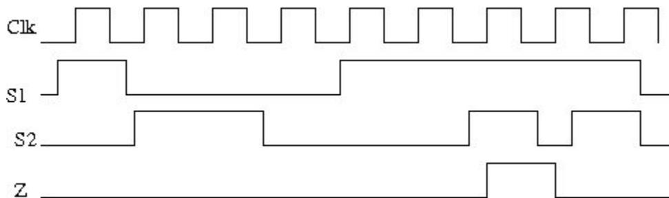
Design a synchronous sequential circuit using D flip-flops that implements the above combination lock. Your circuit should be minimal.
