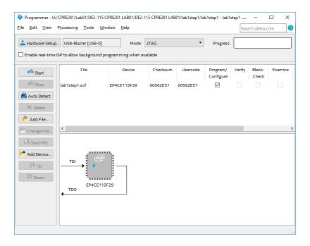
When the green LOAD LED (adjacent to the blue POWER LED) extinguishes, the FPGA will be programmed with your digital circuit. You may now test the behavior of your circuit. The Answer Sheet has a Truth Table for this circuit. Toggle the switches (inputs) and observe the LED (output). Record the results for the circuit's output on the right
