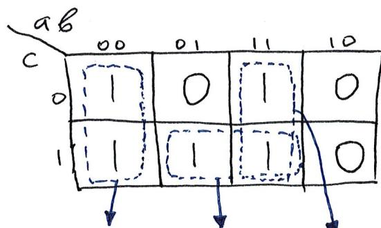
$$f = \overline{a} \overline{b} + b c + a \overline{b}$$
