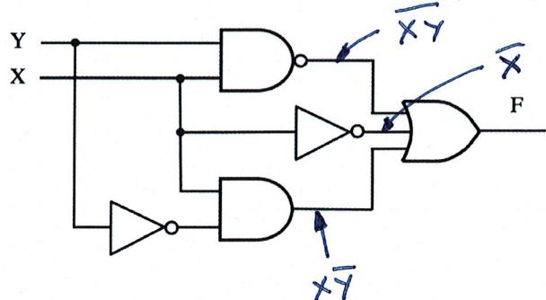
$$F = \overline{X}Y + \overline{X} + X\overline{Y}$$
