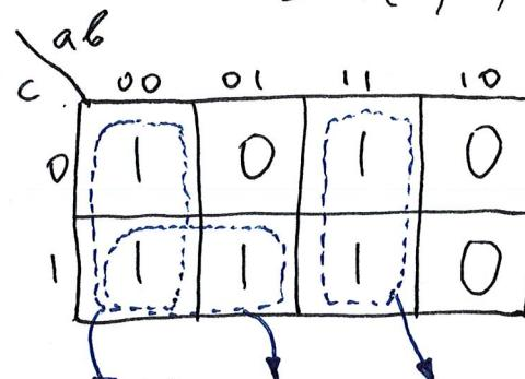
$$f = \overline{a} \overline{b} + \overline{a} c + a \overline{b}$$
