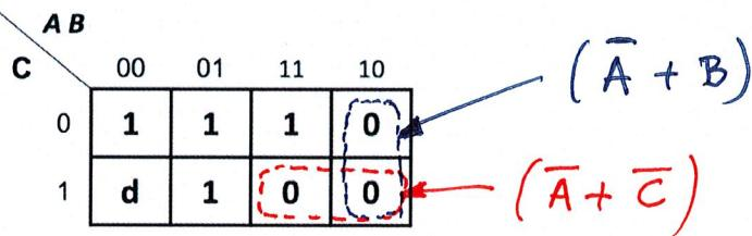
$$F = (\bar{A} + B) \cdot (\bar{A} + \bar{C}) = \overline{(\bar{A} + B)} \cdot \overline{(\bar{A} + \bar{C})} = \overline{\bar{A} + B} + \overline{\bar{A} + \bar{C}}$$
