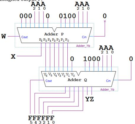
A: What is the expression for outputs W and X in this circuit? Why? B: Describe P, the 7-bit output of "Adder P", algebraically, in terms of A. Note that the output of "Adder P" differs from the left addend of "Adder Q". C: Describe V, the left 7-bit input to "Adder Q", algebraically in terms of A. D: Considering that the output bits Y and Z are ignored by F, describe F algebraically in terms of A.
