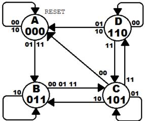
I: Fill in the timing diagram below given the state diagram for a circuit that implements this state diagram using Positive-Edge-Triggered D FlipFlops.
