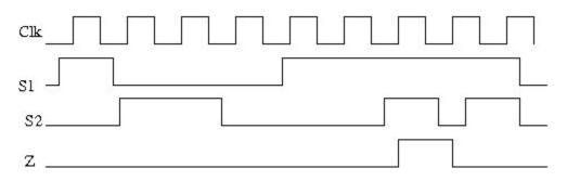
Design a synchronous sequential circuit using D flip-flops that implements the above combination lock. Your circuit should be minimal.
