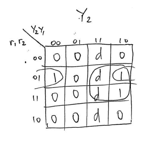
$$Y_2 = r_2 Y_2 + r_1 r_2 Y_1$$
