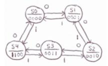
A: Complete the following state diagram with one-bit input F and four-bit input Z ( $z_3 z_2 z_1 z_0$ ). Assume the state variables are V2, V1, and V0. Assume the state assignments are as follows: S0 = 000, S1 = 001, S2 = 010, S3 = 011, and S4 = 100. In the diagram below, the state and output all start at the value 0. The circuit is implemented with positive-edge-triggered flip-flops.
