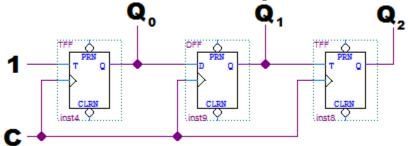
A: What is the counting sequence of this circuit? Assume that the output Q is initially 000.
