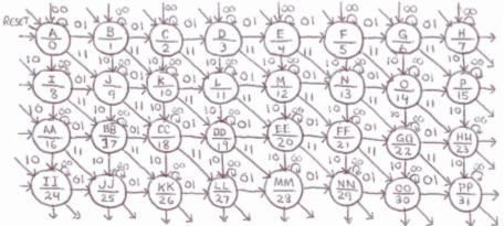
A: What is the minimum number of state variables that can be used to implement this FSM?
