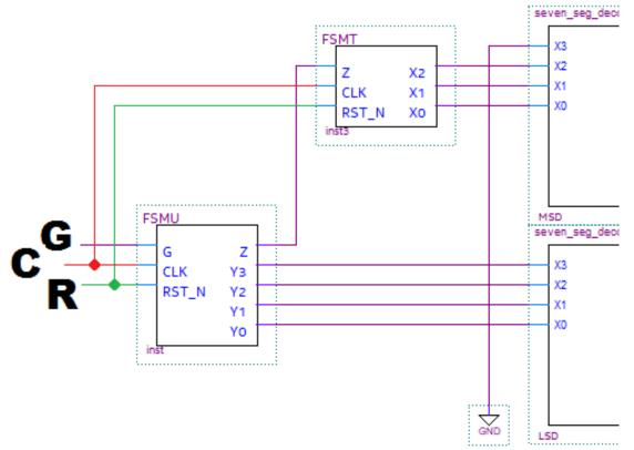
Each FSM shown here has states determined by a sufficient number of positive-edge-triggered DFFs.
