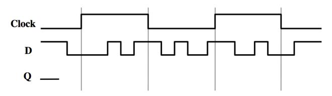
b) Complete this timing diagram a negative edge-triggered T flip-flop. (5pt)
