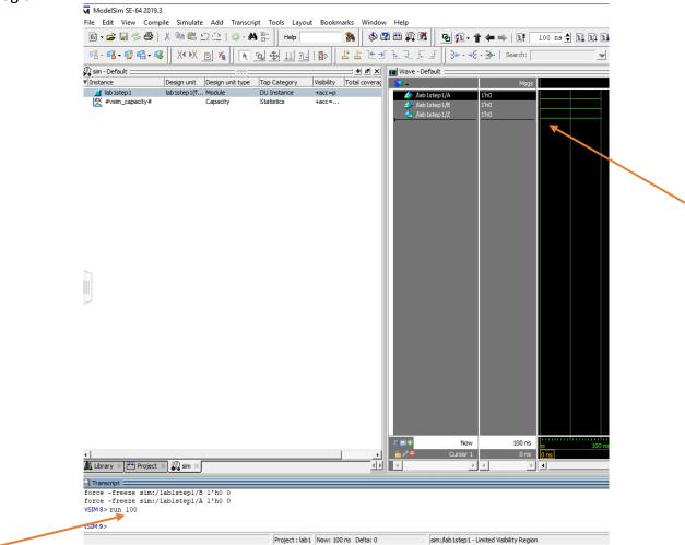
Simulate the output for the other input combinations of A and B by again selecting the inputs and right-clicking to select **Force**. Generate the output waveform by typing **run 100** in the command window. Once the output combinations are generated from all of the input combinations, discuss the results with your TA and have the TA mark their initials next to your answers.
