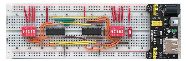
5) Connect the switches to ground using resistors and add the resistors for the LEDs. Because of the complexity of the circuit, we have trimmed the legs of some resistors in these pictures. Yours will be longer. Ensure that the long end of each LED is connected to a resistor and the short end to the – rail.
