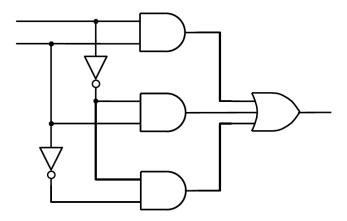
P7. (20 points) Consider the logic function  $f(x, y) = (x + y) \cdot (\overline{x} + \overline{y})$
