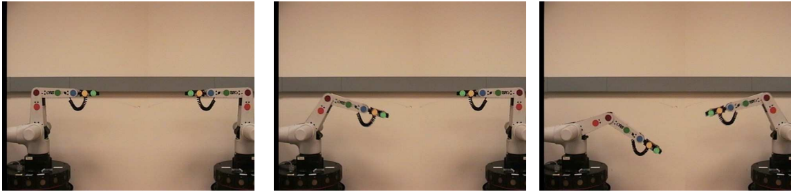
Figure 5.22: Frames from a test sequence with two robots in which the robot on the right mimics the robot on the left. The mimicking delay is 20 frames (0.66 seconds).
