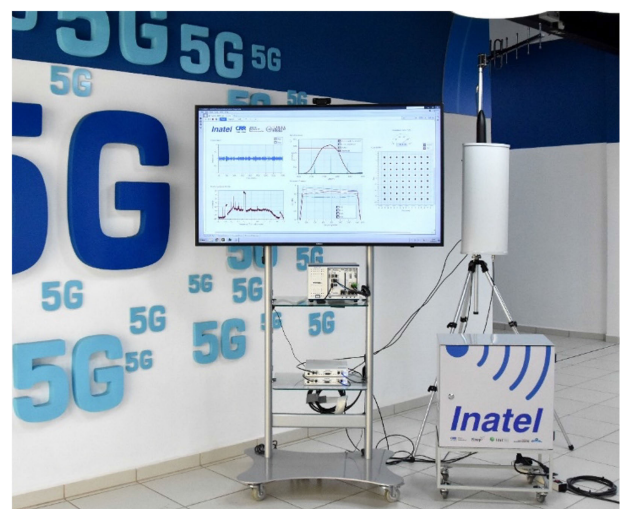
Fig. 15. Prototype of the 5G-RANGE BS.
