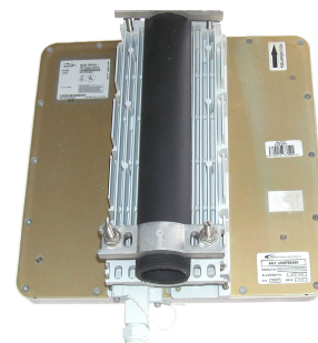
Fig. 17. Alvarion transceiver with massive heat sink fins.
