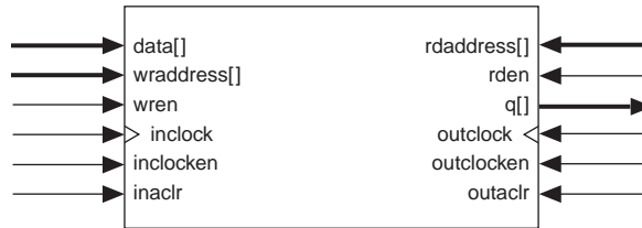
Figure 2-13. Simple Dual-Port & Single-Port Memory Configurations
